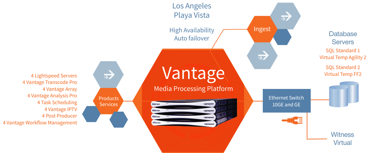
Pop Media Network's Los Angeles Playa Vista IP-networked data center, simplified block diagram
